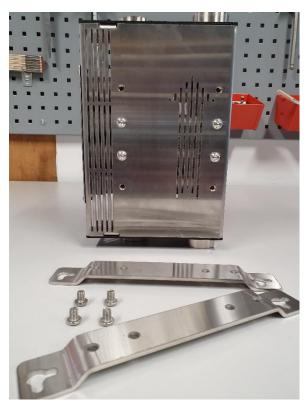
2. Remove up to four screws, two for each bracket. DO NOT remove more than four, as these screws are also a part of how the internal pipings are mounted.
