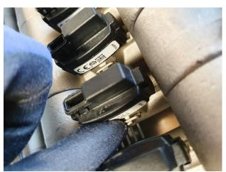
10. Push the locking pin all the way in. You will know that it is all the way in, when it is within the small gap of the hook on the piping.
