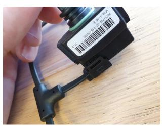
6. Place the sensors, so they rest on the cable, and ensure that the sensors and cable are aligned.
