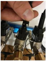
3. Once both sides are released from the 4. Continue doing this for all the sensors you need to remove from the cable.
