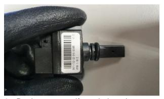
6. Replace sensor if needed, and remount the O ring if it fell off in step 5.
