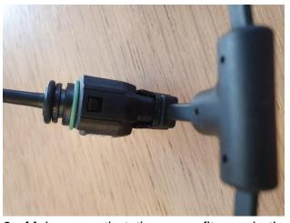
8. Make sure that the snap fits on both sides lock the sensor.
