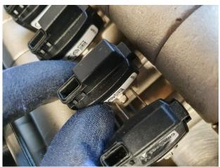
3. Once the pin is pulled out far enough, the sensor is no longer locked in place.
