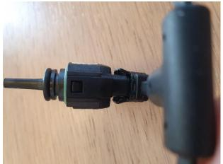
You will know that the sensor is NOT LOCKED in place if the snap fits bend out as shown above
