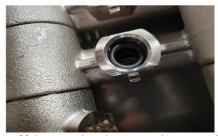
5. Make sure that the sensor is removed correctly. Remove anything from the pipes, like the O ring which commonly gets stuck.
