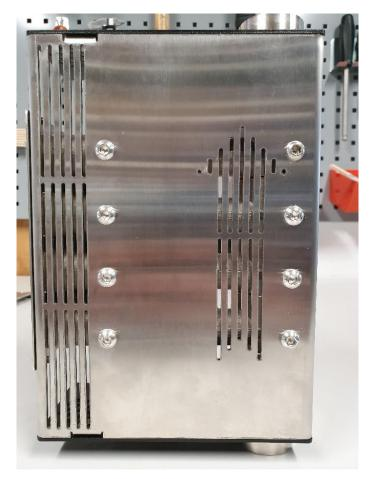
1. The underside of the flosense has screws in place, which can be removed to place the brackets.
