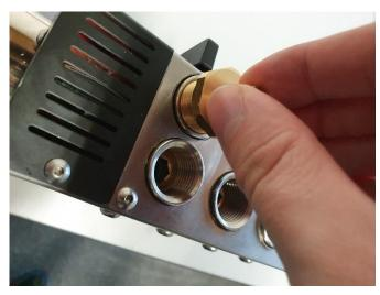
1. Select fittings appropriate for your needs. 2. Insert the fitting in the first channel. It is Remember to have an appropriate O ring on recommended to start with the top row.
