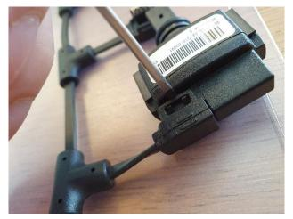
1. In order to remove the cable, you will need a small tool, such as a screwdriver in order to lift the snap fits holding the sensor.
