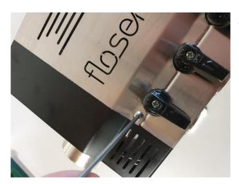
2. Remove all the screws with an Unbrako key
