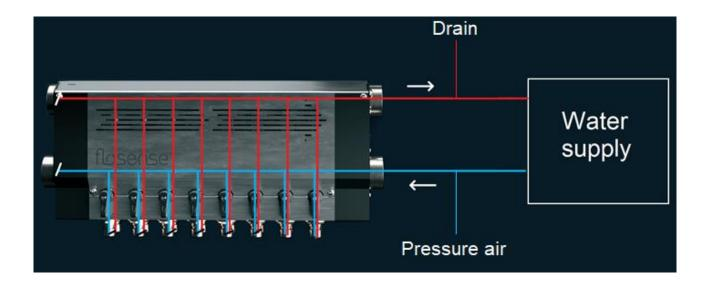
Warning: if pressurized air supply exceeds 0,5 bar, the flow sensors may be damaged due to extreme purge speed.
