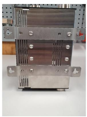
3. Mount the brackets by using the same screws which were just removed. Beware that the bracket should be mounted so the holes at the ends point "upwards" as on the picture. If the holes are pointing "downwards", then the manifold can still be mounted, if you turn it upside down.
