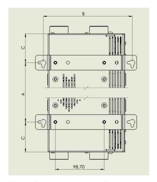
The position of the holes for the bracket can be seen in the figure above, and the dimensions for each model can be seen in the table below.
