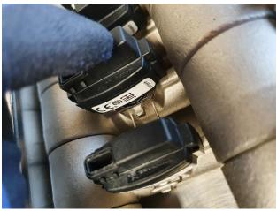
8. When the sensor is placed vertically, it can be pushed down into the piping
