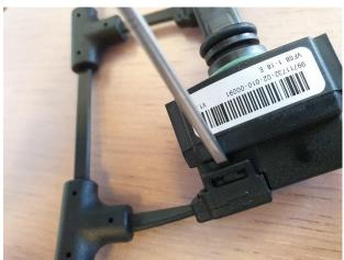
2. Lift the snap fit gently, so as not to break it. Once it bends slightly, you will know that it has released. Do this for both sides of the sensor.
