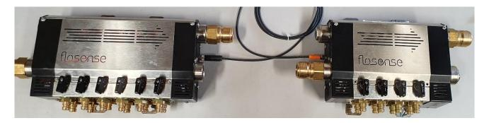
The right manifold is the first manifold and is the one that should be connected to the Flosense display on the right side of the picture. On the left side of the right manifold, the cable is connected to the M8 connector (orange connector). The cable is then connected to the left manifold, on its right side (black connector).
